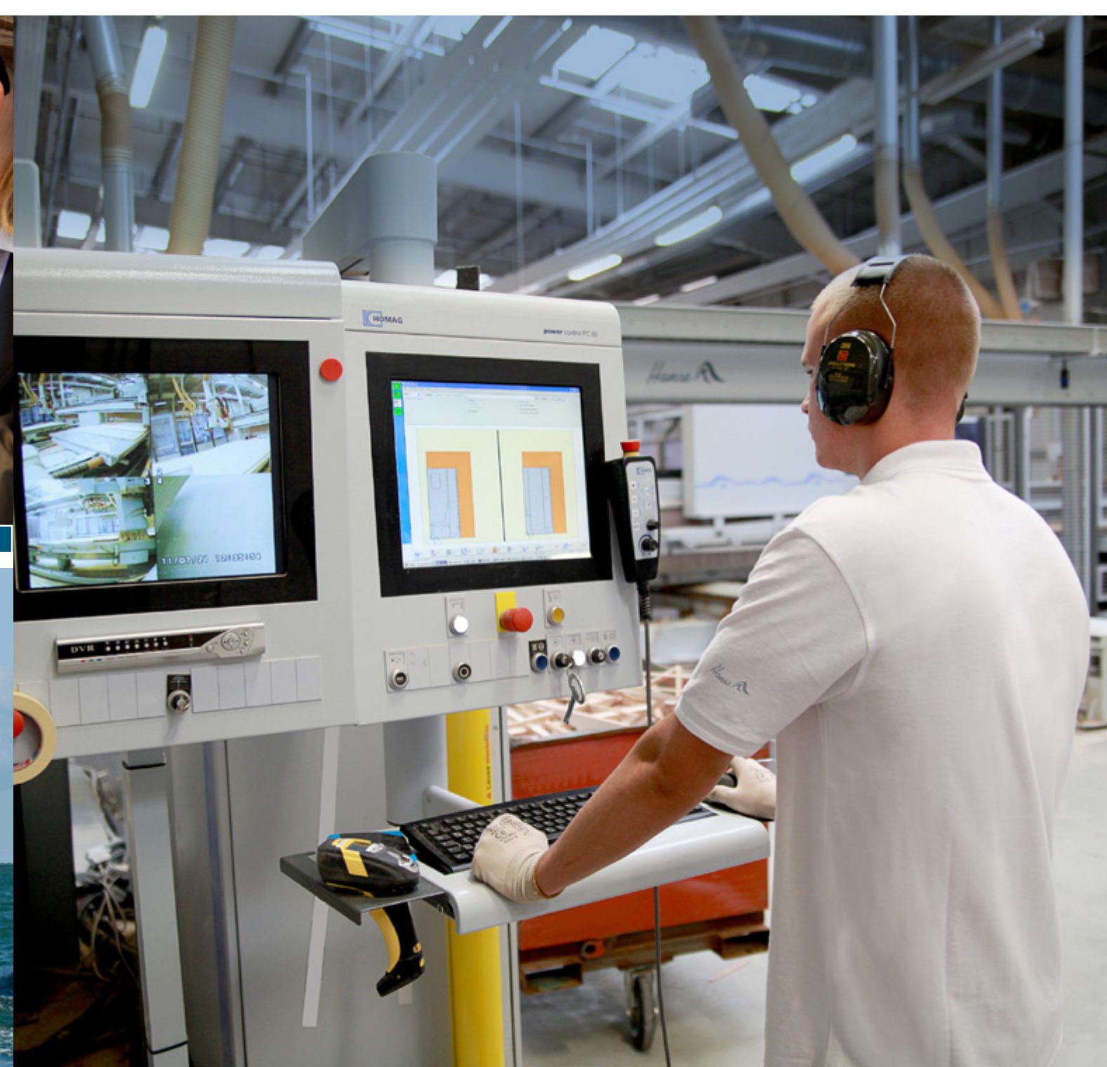
4 Before our carpenters build the interior of a HANSE 345, wood panels are prefabricated using computer control.
