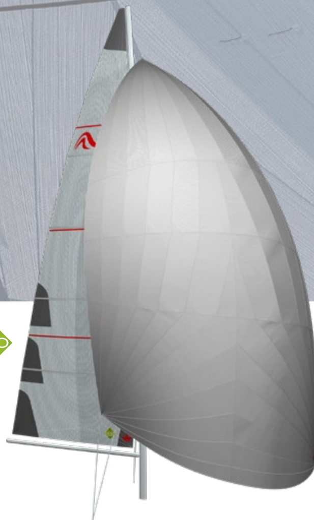
Conventional main sail Material: Elvstrøm SPS Laminate Layout: Triradial
