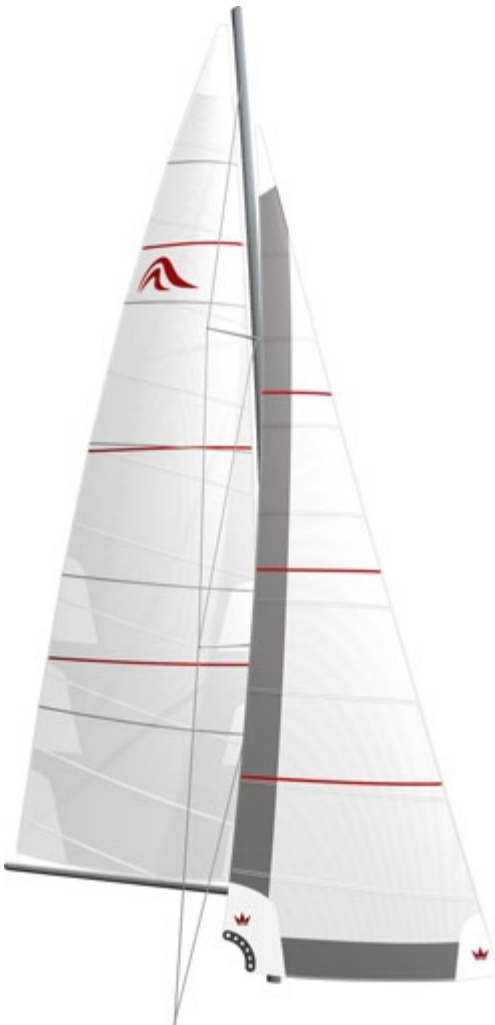
Conventional mainssail Material: Elvstrøm Blue Water Dacron white Layout: Cross cut
