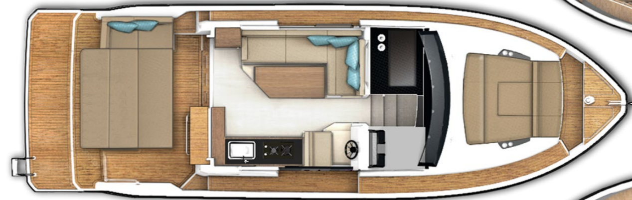
Main deck option with cockpit table to be transformed into sunpad and extended bathing platform
